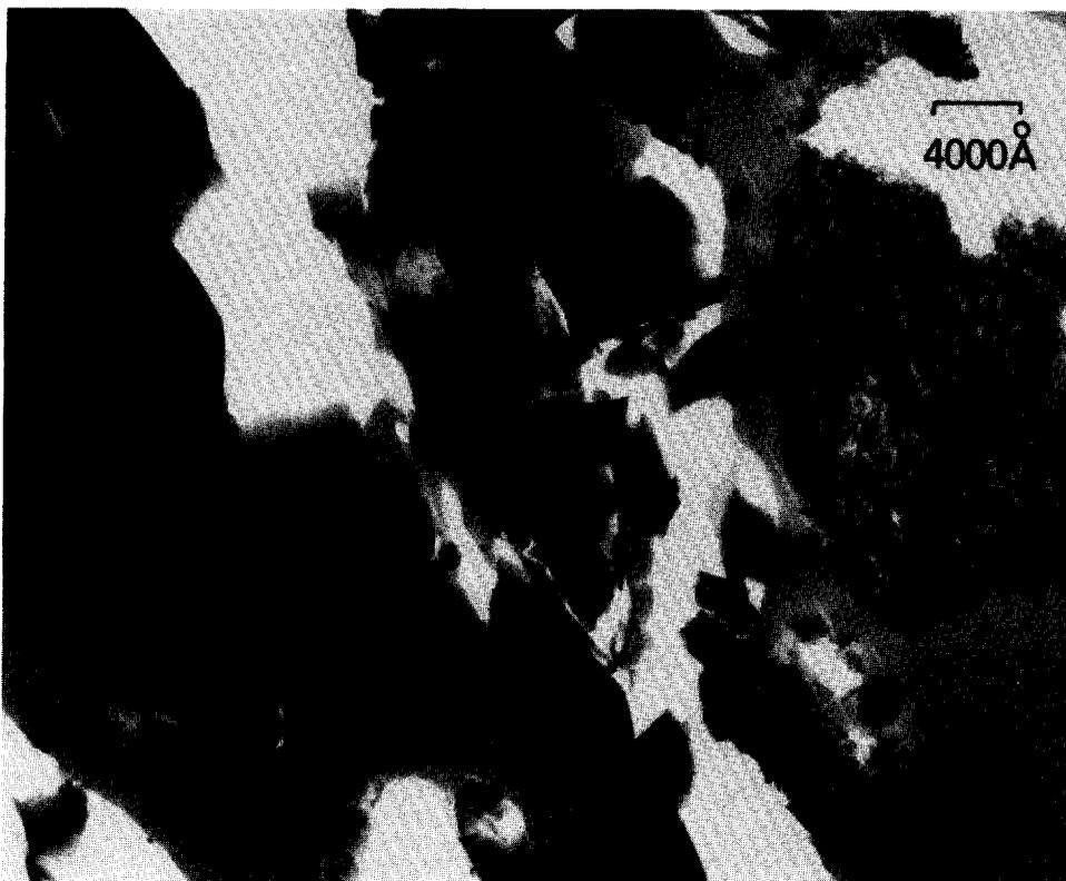
FIG. 8. Thin section TEM of fresh mordenite.
